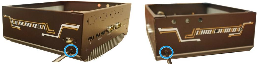
5. Separate the two I/O panels.
