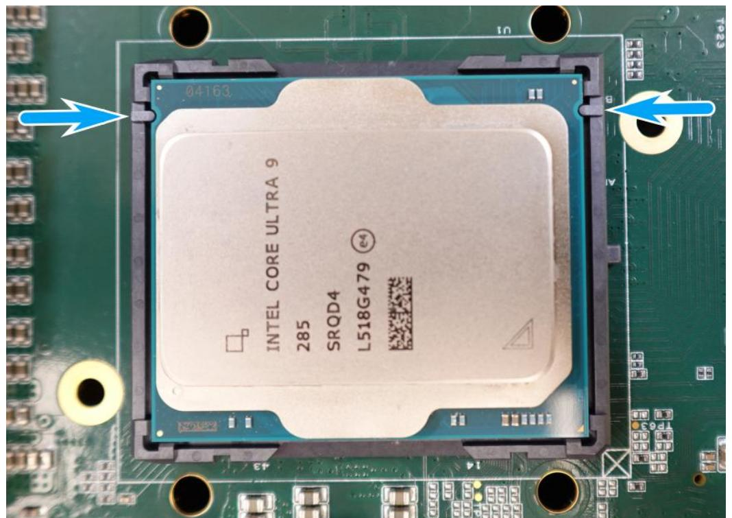
12. Make sure all thermal pad residues have been cleaned on both sides of the retention
