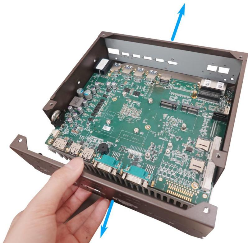
6. Remove the eight screws indicated below. Please use a hex-bolt socket for the stand-off indicated in **red**.
