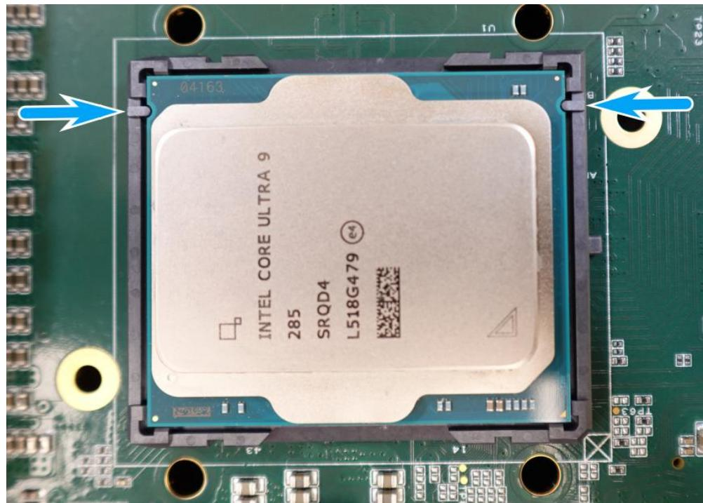
10. Locate the CPU retention bracket (holder) from the accessory box. Place the retention bracket on the CPU and hold it in place. Make sure the indicator triangle engraved on the CPU's integrated heat spreader (HIS) and the triangle indicator on the retention bracket are positioned in the same corner (indicated by **blue circles**).
