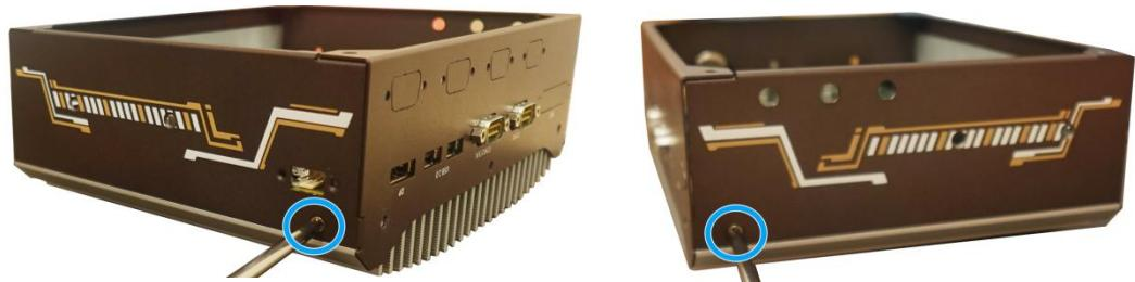
19. Secure the hexa-screws on both I/O panels.
