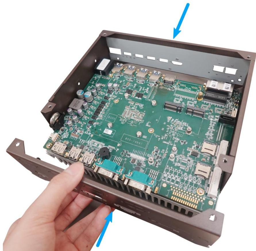
18. Secure the screw indicated on the side panels.
