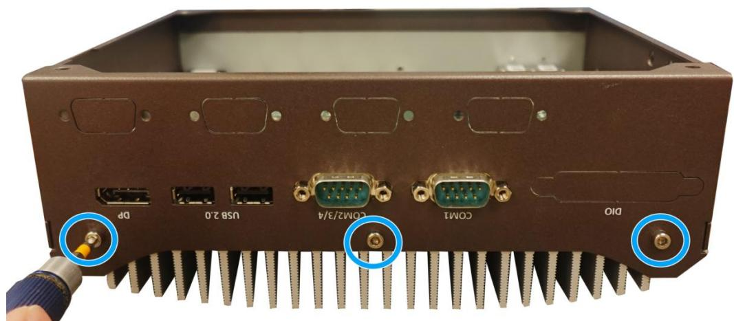
4. Remove the screw indicated on the side panel.
