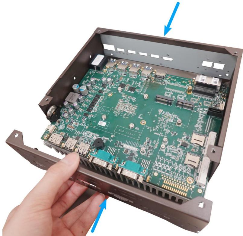
13. Secure the screw indicated on the side panels.
