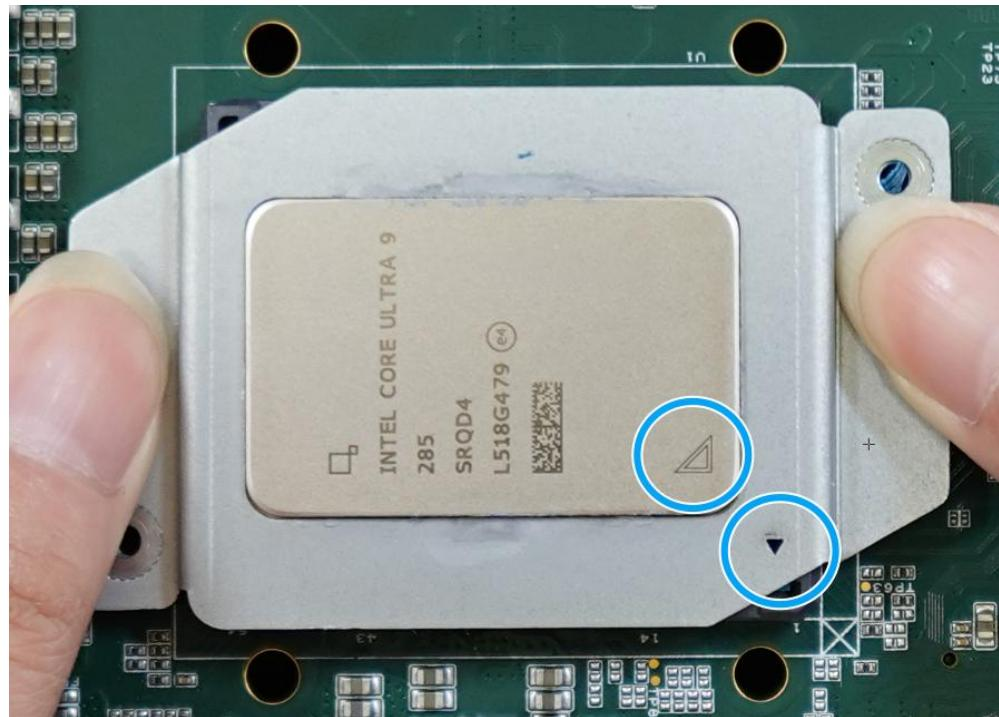
13. Turn the motherboard around while holding the CPU retention bracket in-place, and secure the bracket by tightening two M3 P-head screws on the other side of the motherboard.
