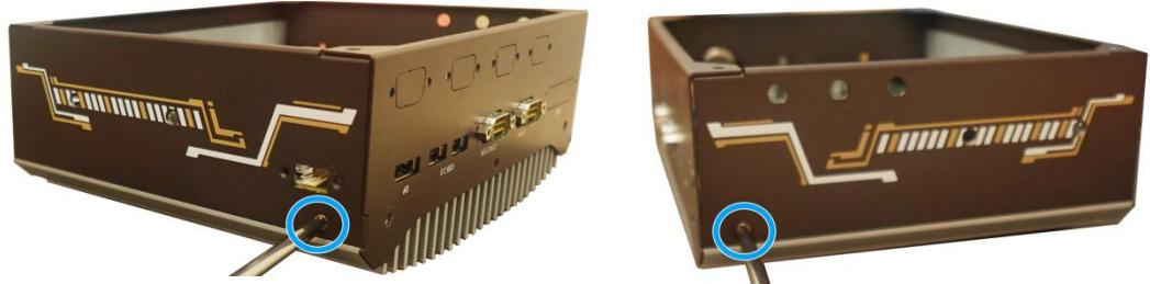
5. Separate the two I/O panels.
