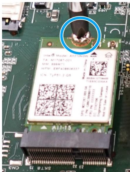
6. Clip on the IPEX-to-SMA cable to the module and secure the antenna to the side panel.
