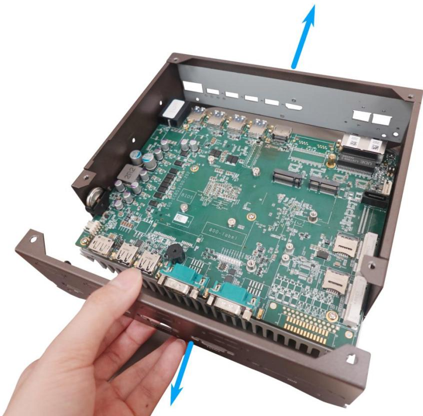
6. Remove the screws indicated on the motherboard. Please use a hex-bolt socket for the stand-off indicated in red.
