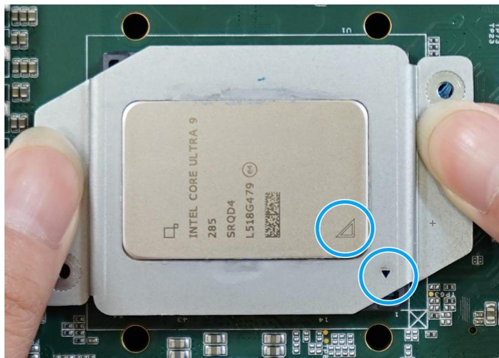
11. Turn the motherboard around while holding the CPU retention bracket in-place, and secure the bracket by tightening two M3 P-head screws on the other side of the motherboard.
