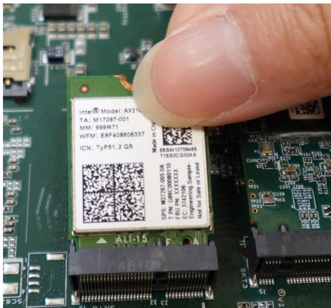
5. Gently press down and secure the module with an M2.5 P-head screw.
