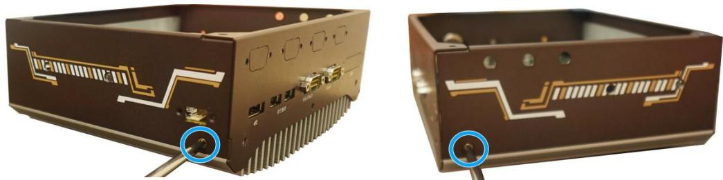
14. Secure the hexa-screws on both I/O panels.
