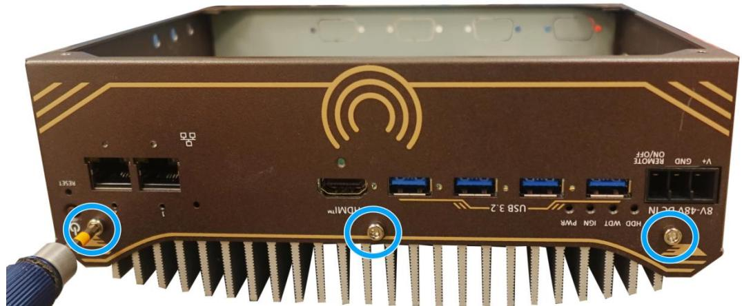
3. On the I/O panel with the DisplayPort, remove the hexa-screws indicated below.
