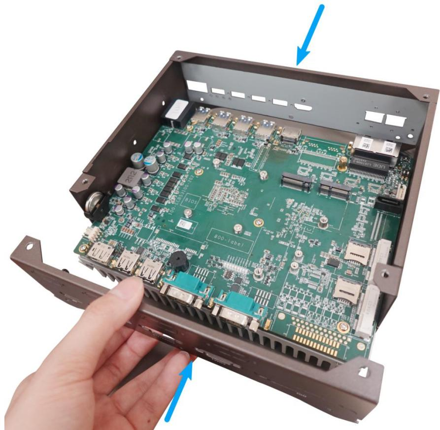
16. Secure the screw indicated on the side panels.
