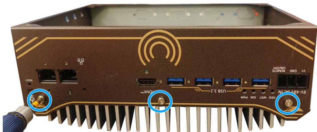
3. On the I/O panel with the DisplayPort, remove the hexa-screws indicated below.
