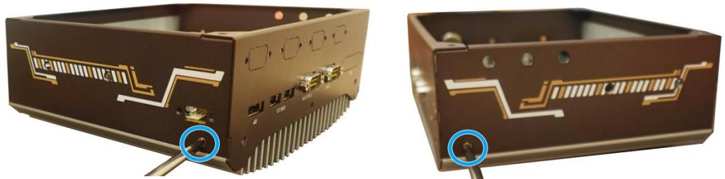
17. Secure the hexa-screws on both I/O panels.
