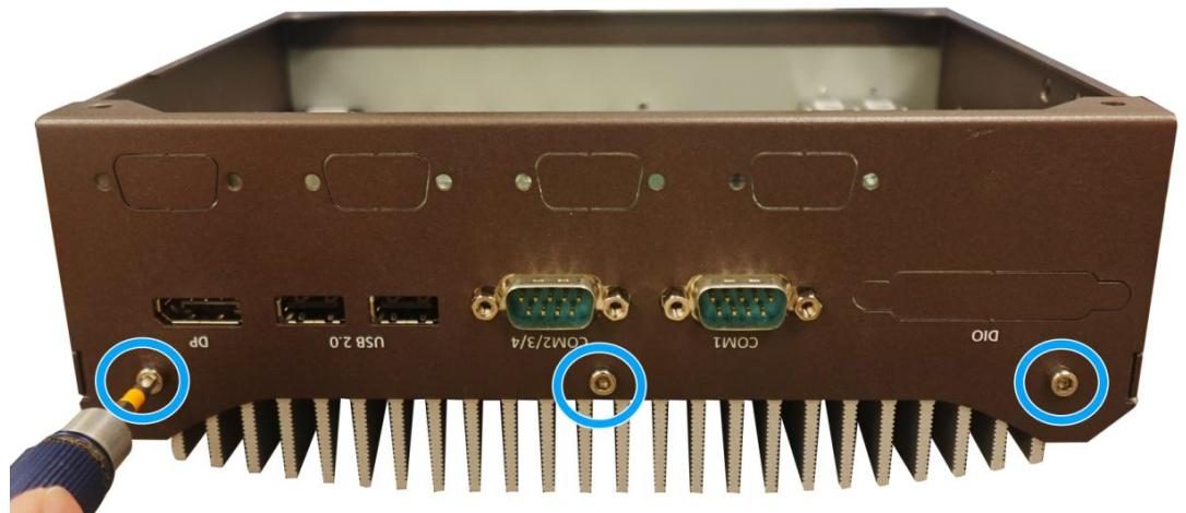
4. Remove the screw indicated on the side panels.
